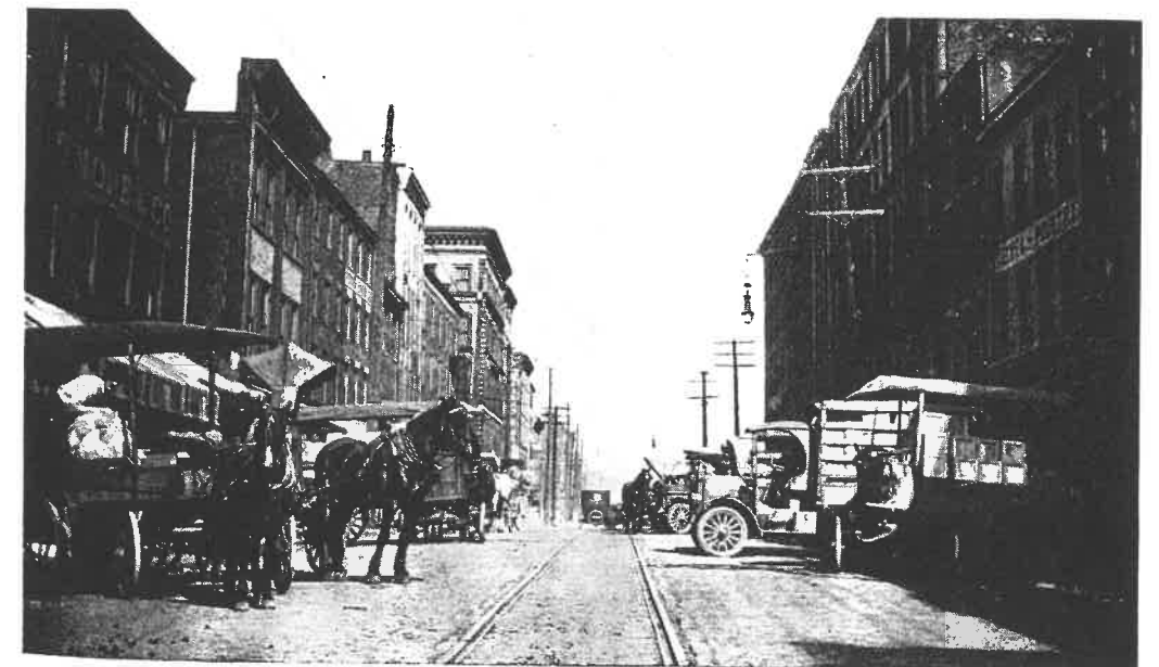
FRONT, SECOND AND THIRD STREETS TRUCKING CONGESTION Tail loading often leaves only one clear traffic lane
