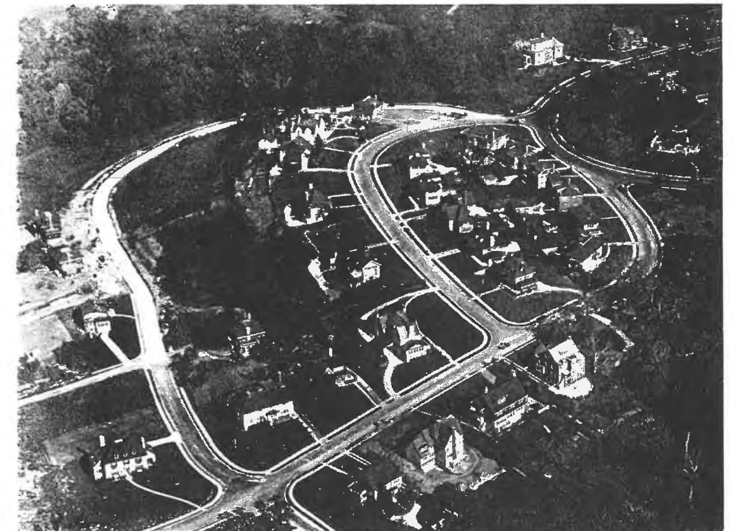
AVON HILLS SUBDIVISION (Courtesy of Mr. Morgenthaler) A model for the fitting of streets and lots to topography.
